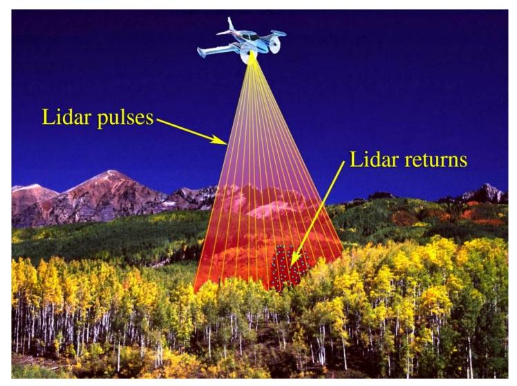
Caption: A LIDAR instrument principally consists of a laser, a scanner, and a specialized GPS receiver. Airplanes and helicopters are the most commonly used platforms for acquiring LIDAR data over broad areas.
